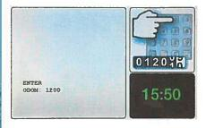
The PV200 uses text and graphics to prompt drivers to enter information such as vehicle number, driver number and odometer reading.
